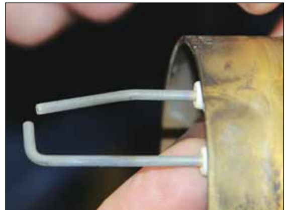
Top —Part of the secret to a clean burn is the tiny orifice in the spray nozzle through which diesel is injected at 300 psi (2.1 N/mm 2 ) and its anti-dribble valve that prevents post-shutdown smoking and fouling. The atomization of fuel coupled with a conventional furnace blower and a large ignition spark gap ( bottom ) permits a near-complete burn.
