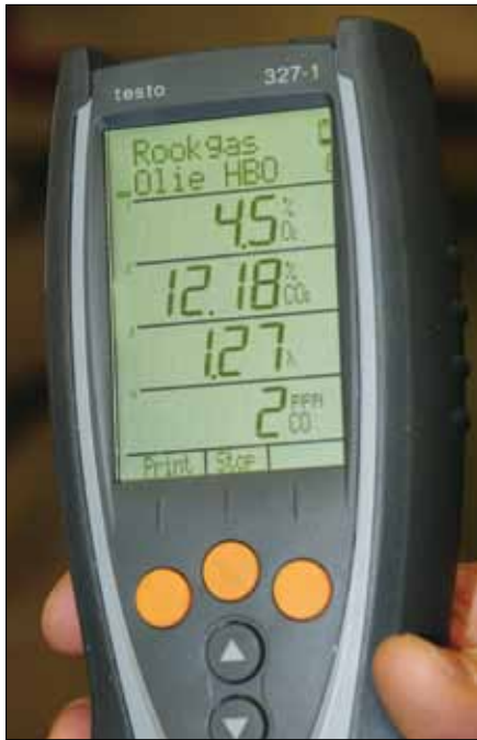
Readings of exhaust from an operating heater show carbon monoxide levels at a scant two parts per million.
