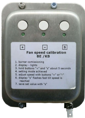
Controller board, with the description of the fan speed adjustment
